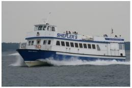
to accommodate 210-passengers, being propelled by four Hamilton Jet water jets. The new jet-propulsion means a shorter and quieter trip for passengers.
