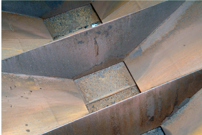
Detail of hogbacks and conveyor tunnel gates on the Wilfred Sykes . Photo by Roger LeLievre
