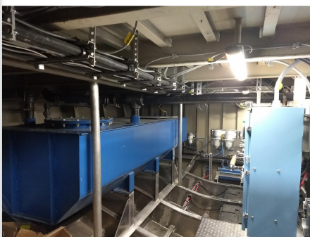
One of the 900 gallon fuel tanks and the electrical panel, photo by Brendan Falkowski
