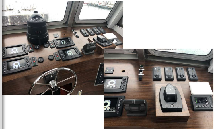
Modern helm controls aboard the William Richard . The computer-mouse appearing control at center can be used to steer the ship and pivots 360 degrees. Photo by Chris Shepler
