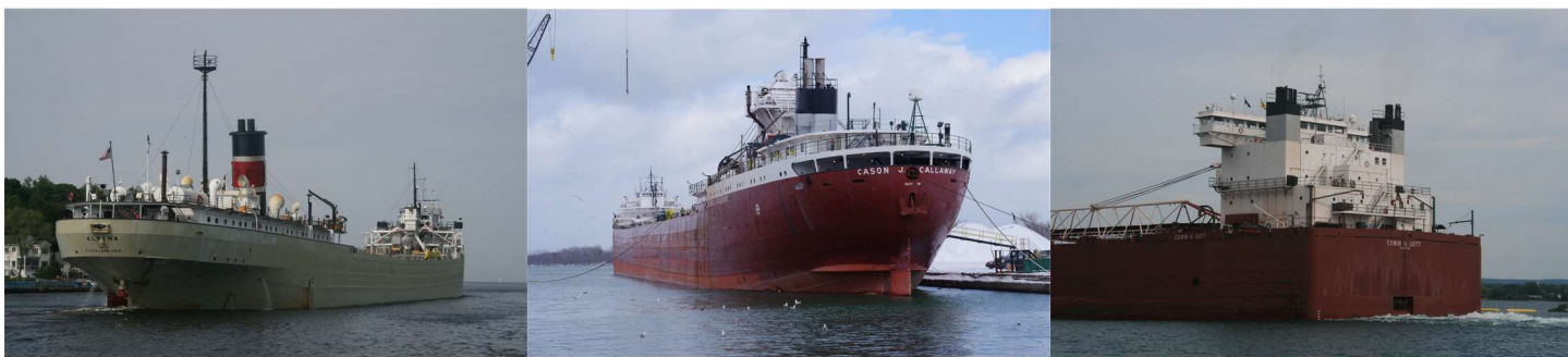
Counter – elliptical stern on Alpena .; Cruiser stern on Cason J. Callaway . Photo by Isaac Pennock; Transom – raked stern on Edwin H. Gott . Alpena and Gott photos by Brendan Falkowski
