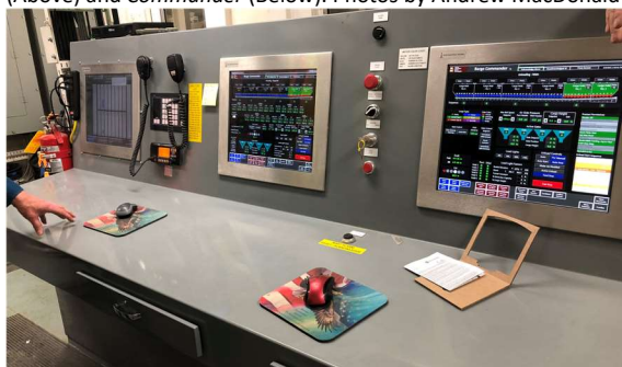
Comparison of unloading controls onboard St. Marys Conquest (Above) and Commander (Below). Photos by Andrew MacDonald
