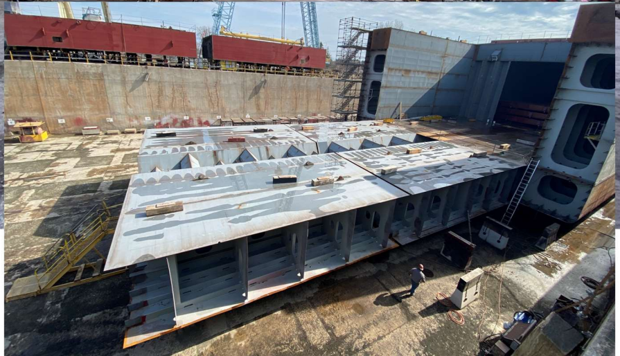
Two forward keel blocks added to the hull
