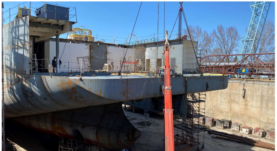
Stern view of aft deck under construction
