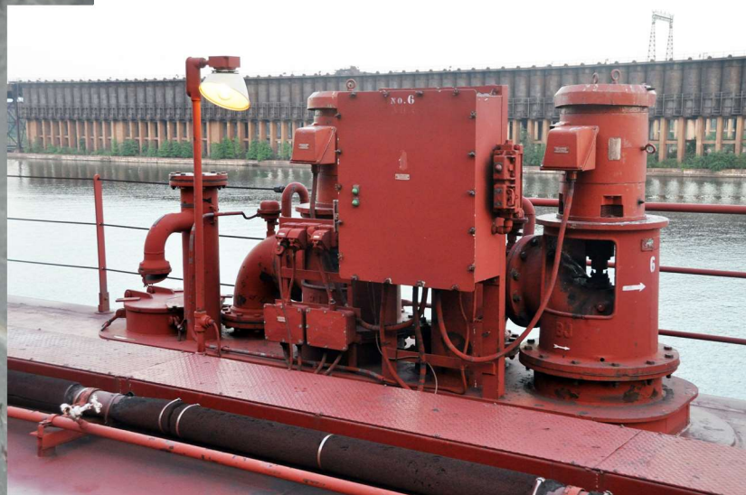
(Above) Ballast pump on the spar deck of the Stewart J. Cort . Photo by Roger LeLievre (Left) Water is discharged from the St. Marys Challenger , 2009. Photo by Roger LeLievre
