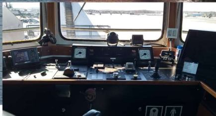
View forward inside the pilothouse of the tug Dirk S. VanEnkevort . A chair is in the foreground. The tug is steered by a joystick at the center of the picture. Photo: Brendan Falkowski
