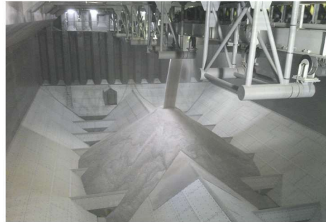
Travelling reversible shuttle conveyor loading salt into the vessel cargo hold. System designed and supplied by EMS-Tech Inc. Photo: EMS-Tech
