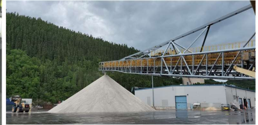
80meter boom conveyor discharging salt to a pile at a rate of 5,450mtph. This particular boom conveyor is fitted with a 26meter shuttling section to support to support the control of the pile height when discharging. Photo: EMS-Tech
