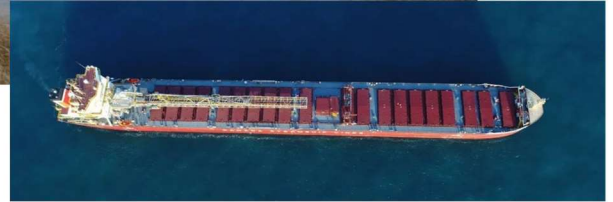
(Above) MV Nukumi being loaded with salt at a rate of 4,000mtph to the fixed SPL hopper. (Below) MV Nukumi – Laker Self-Loading / Self-Unloading vessel. 26,000dw. Single Point Loading hopper at mid-ship location. Both photos: EMS-Tech
