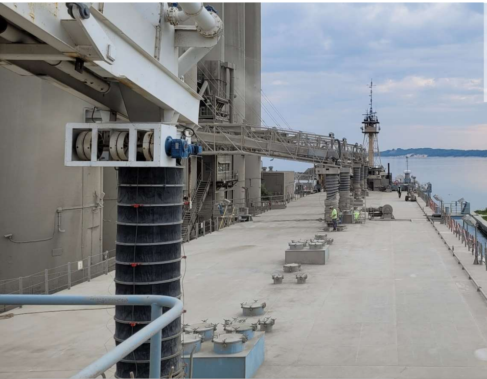
(Main) Commander loads from the chutes at Charlevoix. The loading scuttles are visible on the centerline of the spar deck; (Inset, Top-Bottom) McKeil Spirit utilizes vertical screws and a pneumatic system to unload. Photos: Brendan Falkowski; Schematic of a Fuller-Kinyon Cement Pump, cement enters through the hopper on the right and is pumped out the pipe on the bottom center. Photo courtesy of Nick Hunter.
