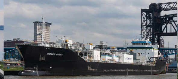
(Main) Commander loads from the chutes at Charlevoix. The loading scuttles are visible on the centerline of the spar deck; (Inset, Top-Bottom) McKeil Spirit utilizes vertical screws and a pneumatic system to unload. Photos: Brendan Falkowski; Schematic of a Fuller-Kinyon Cement Pump, cement enters through the hopper on the right and is pumped out the pipe on the bottom center. Photo courtesy of Nick Hunter.
