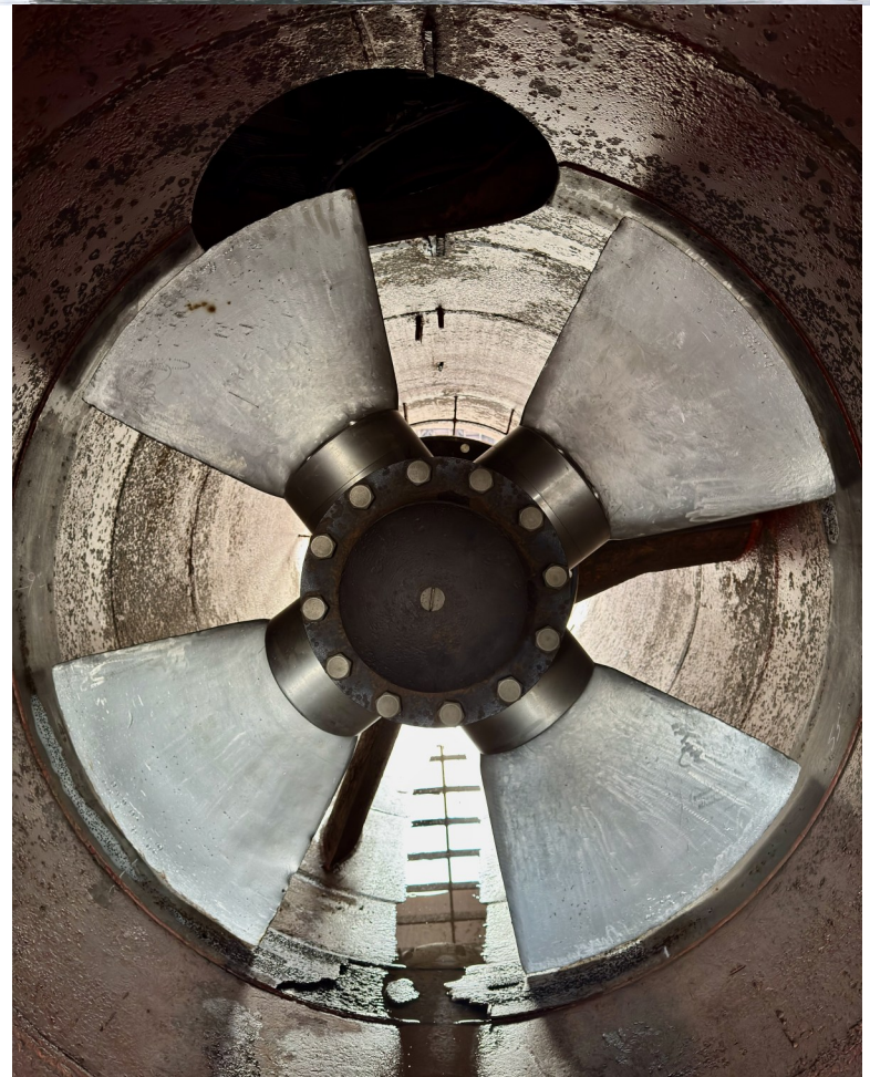
(Top): Tugs assist the SAM LAUD while she uses her bow thruster in the Trenton Channel, September 28, 2023. Photo: Sam Hankinson; (Below): View of the bow thruster tunnel onboard the PHILIP R. CLARKE, September 17, 2024. Photo: Daniel Lindner
